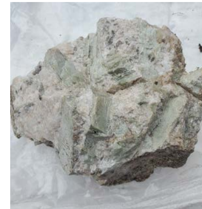
RIGHT: Grab sample from showing significant spodumene crystals
